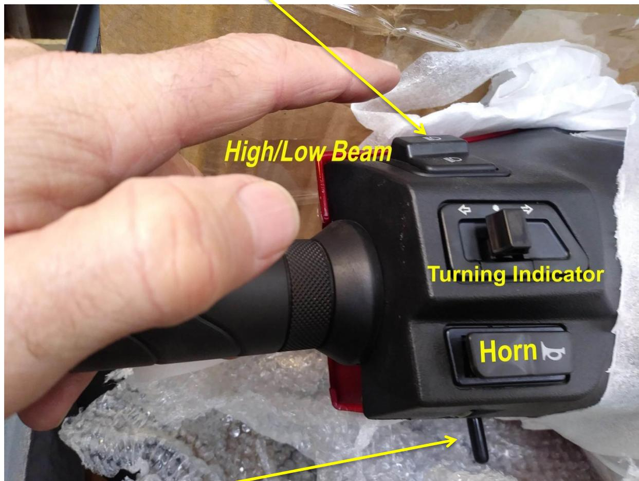
**Brake Lock Rod:** While squeezing left brake, push rod up to lock. Squeeze brake to release. Will prevent scooter from rolling on hill when parked.
